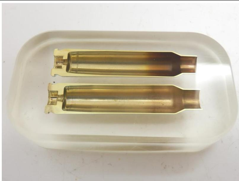
**Figure 2.1 Typical mounted and polished cases for examination**
