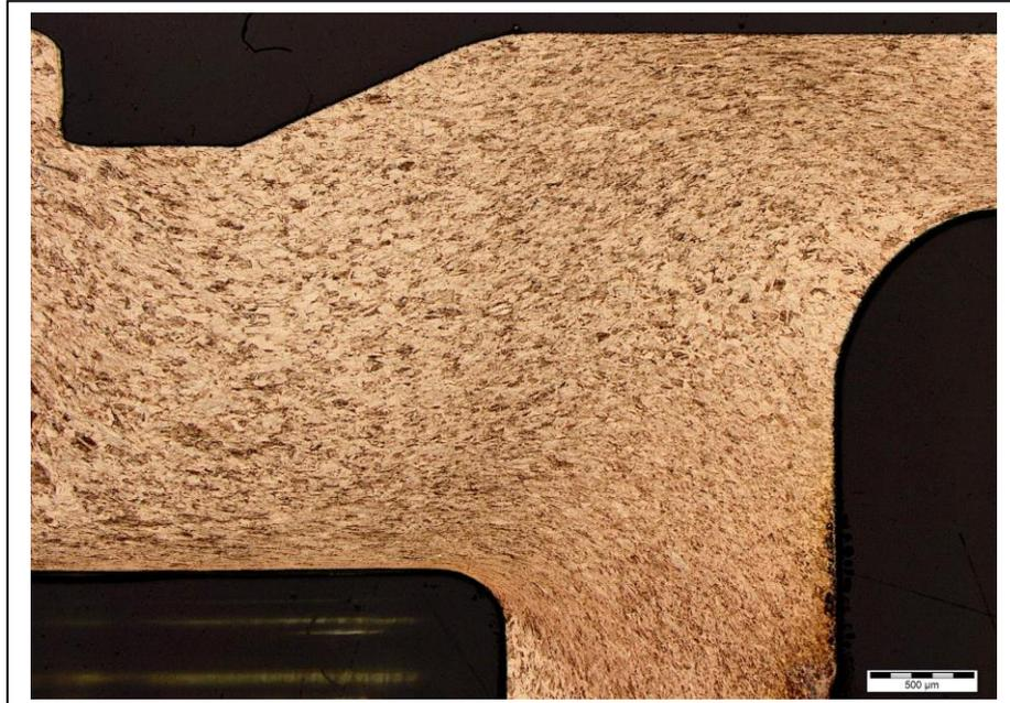
Figure 3.4 Microstructure in the head of the 223 case, 25x
